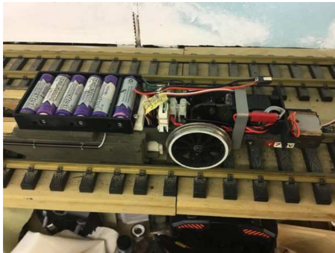
The 6 cells AA NiMH (7.2 volts) sit over the Rx. The ESC sits between the frames under the motor. The motor running sound card sits vertically just in front of the driving wheels.
